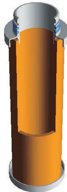
Cross section of the SB prefilter
